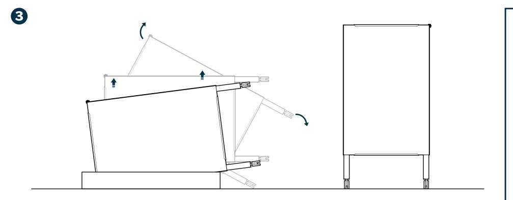
After locking the casters, with one person on each side of the board, lift it up and rotate it into a vertical position. Gently place the feet on the ground.
