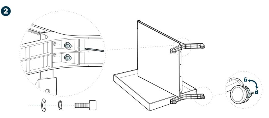
Next, use the provided T-Handle and hardware to attach the feet to the receiving pegs. Place one lock washer on the screw followed by one washer, then screw into the bottom of the feet. Repeat until all four screws are in place. Lock the casters to keep the wheels from rotating.
