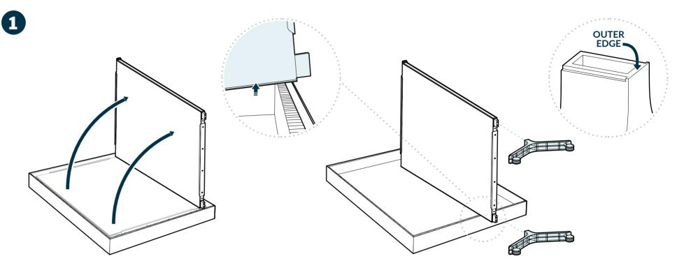
After unboxing, with one person on each side of the board, tip the board upright onto its side. Raise the bottom end of the board to rest on the edge of the box. Align the outer edge of each foot with the outer sides of the board, then slide the feet onto receiving pegs on the bottom of the board.
