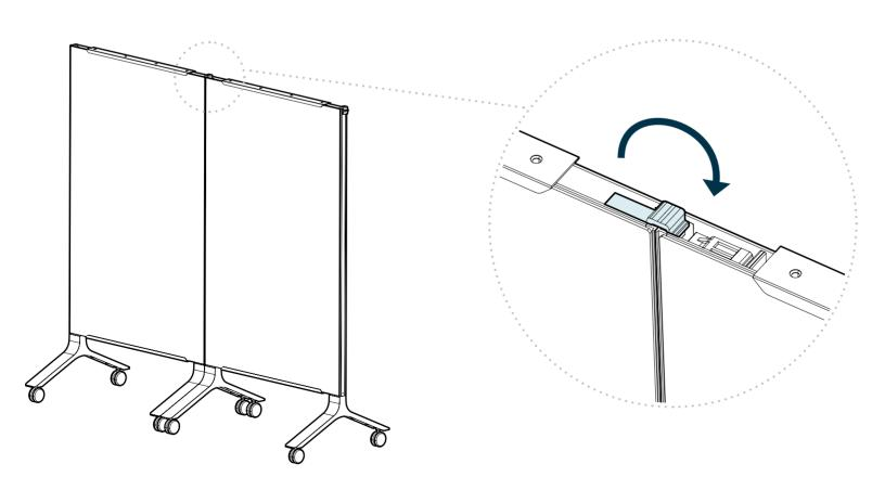
To connect two or more boards together, align the boards side by side and flip the plastic connector on one board over to latch onto the top edge of another board.
